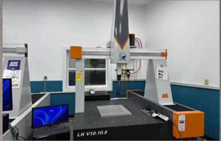
LK Metrology V10.10.8 CMM, Renishaw PH10M Probe
