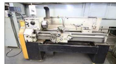
LATHE: LeBlond Makino Regal Servo Shift Lathe 18" x 56" with 2 Axis DRO
