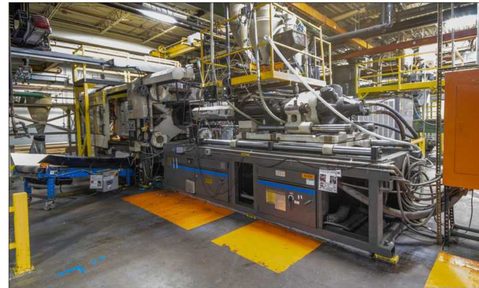
INJECTION MOLDER: Cincinnati 850 Ton Model VH850-140 Injection Mold Machine with Wittman Robot, 107.8 oz Shot, 46" x 37" Btwn. Posts, 58" x 56" Platen, 62" Max. DL, Knock Outs, Mold Vision System installed 2018
