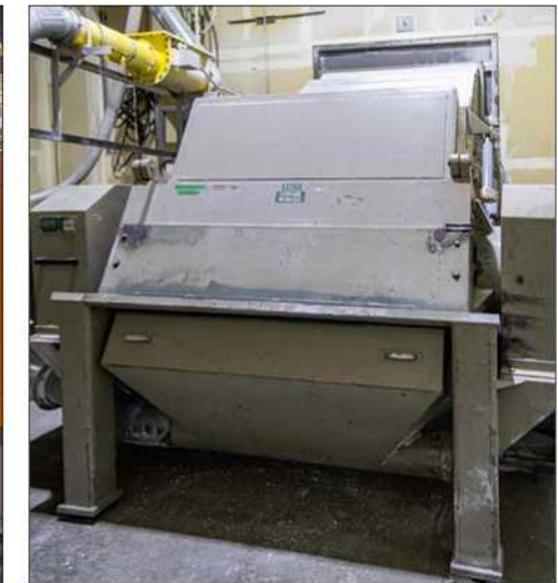
PLASTIC SUPPORT EQUIPMENT: Conair Plastic Granulator / Grinder Model LC 56, 28" Blades, Screen 5/8", 75 HP
