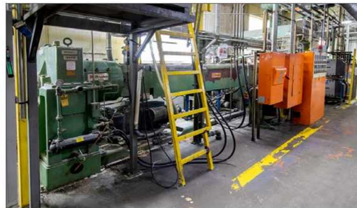
EXTRUSION LINES: (2) Prodex Sheet Extrusion Lines, One 6" and One 4.5", Both Have 3 Roll Calender, Puller with Trimmers, Wysong Shear and Stacker, Extruder
