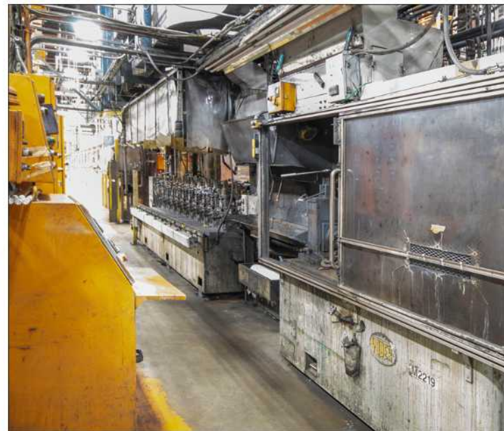
TUBE MILL & STRETCH REDUCING MILL: Yoder Tube Mill and Stretch Reducing Mill-DE Yoder Uncoiler, Shear End Welder, Kent Horizontal Floop, 5 Stand rafted Forming Stand, ERW Welder, Yoder rafted 10 Stand Sizing and Reducing Mill, Annealing Line, Nitrogen Atmosphere Coolant Tube, Yoder 2 Spool Rewinds and Cut Off
