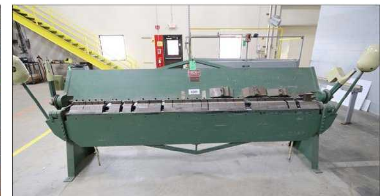
BRAKE: Chicago Dreis and Krump Finger Brake 14 gauge x 10'
