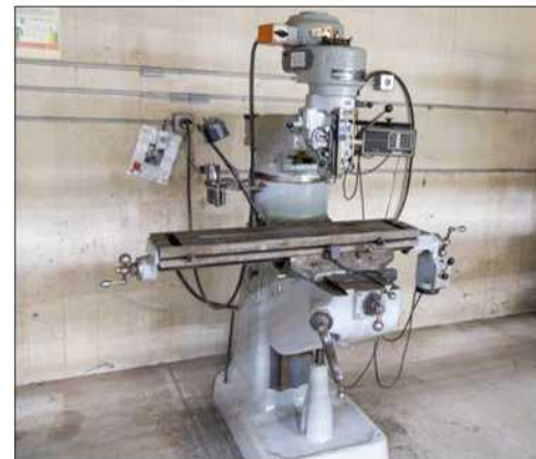
MILLING MACHINE: Bridgeport Vertical Mill 9" x 48" Table, 2 Axis DRO, Auto Feed
