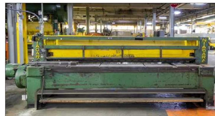
SHEAR: Niagara Power Squaring Shear 3/16" x 126" Capacity Cat# 710-B
