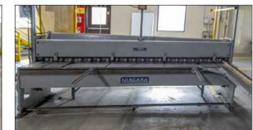
SHEAR: Niagara Power Squaring Shear 3/16" x 126" Capacity
