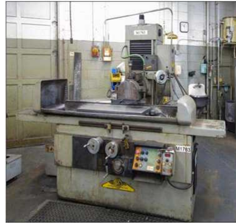
GRINDERS: ELB Schliff Surface Grinder 14" x 34" Magnetic Chuck, Auto Feed
