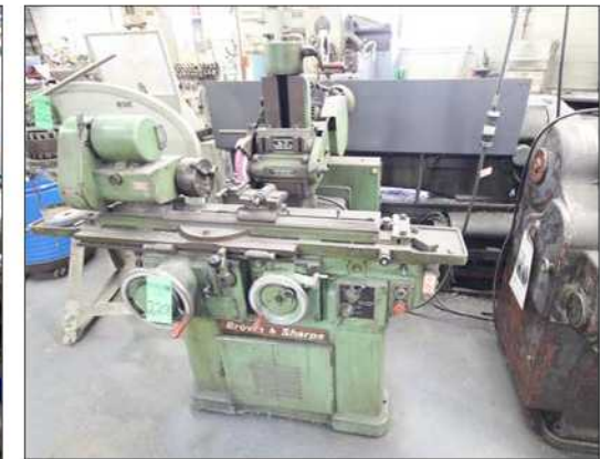
GRINDERS: Brown and Sharp 618 Micro Master Surface Grinder, 6" x 18" Magnetic Chuck, Auto Feed
