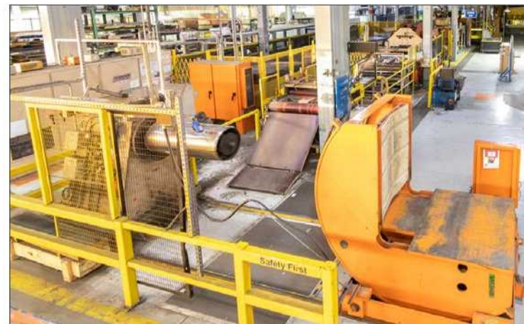
Strilich Line Consisting of- Coil Car Tipper 20,000 lb Cap., Strilich 20,000 lb x 48" Uncoiler, Squaring Guides and Servo Feed, Bradbury 75 ton 4 Post Press (7' x 4'), Pinch Roll and Flying Shear, Inspection and Stacker, Pallet Stuffer, Outfeed Conveyor, Pallet Roll Over Unit
