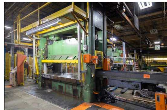
Pacific Hydraulic Press 200D-1036 200 Ton, 36" x 123" Bed, 9 SPM
