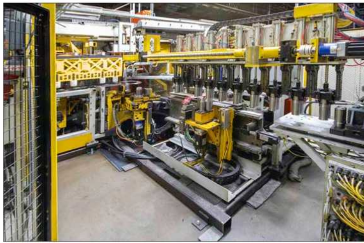
CNC TUBE BENDER: CNC Tube Bender Cell (M-6941), Bends 15 to 20 3/16" Refrigeration Tubes at a Time with Robot Unloader/ tacker
